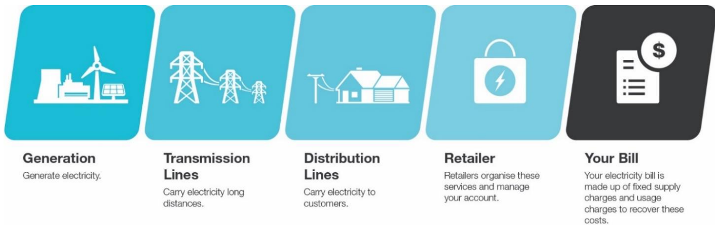
Figure 5 - Stages of charges of an electricity bill
